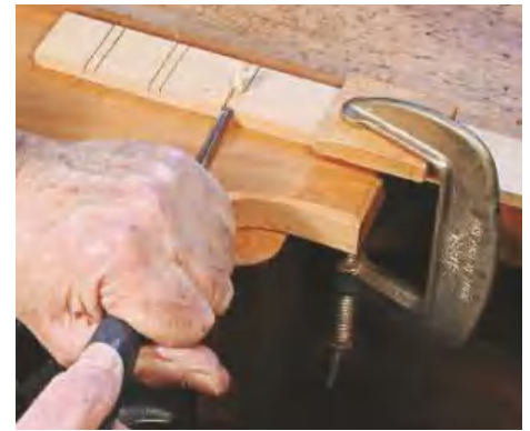
▲ Pic.6 This simple jig holds thin stock securely when making paring cuts
